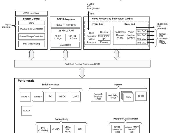
Figure 1-1. TMS320DM643x DMP Block Diagram
